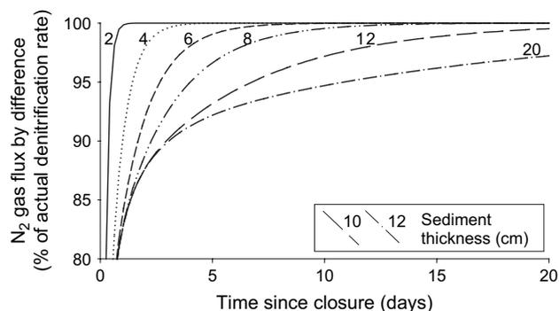
Fig. 4. Modeled denitrification  $N_2$  flux (determined with anaerobic control incubations) from sediments of various thicknesses. Calculated fluxes from thicker sediments are lower because of retention of denitrification-derived  $N_2$  in sediment porewater.
