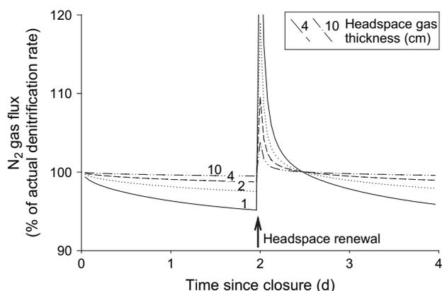
Fig. 6. Modeled  $N_2$  fluxes during headspace renewal. After an initial off-gassing preincubation, the chamber was closed (days 0–2), headspace was renewed (arrow), and chamber was closed again (days 2–4; as in Seitzinger, 1988 and others). A sharp increase in  $N_2$  flux results because the sediment–water concentration gradient increases when headspace gas is replaced by low- $N_2$  gas. Fluctuations in  $N_2$  flux are larger for small headspaces.
