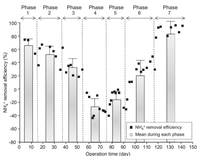
Fig. 4. Ammonium ion removal efficiency in the co-digestion experiment using the upflow anaerobic sludge bed reactor. Phases are described in Table 2. Means and standard deviations for each Phase are indicated by the vertical bars.
