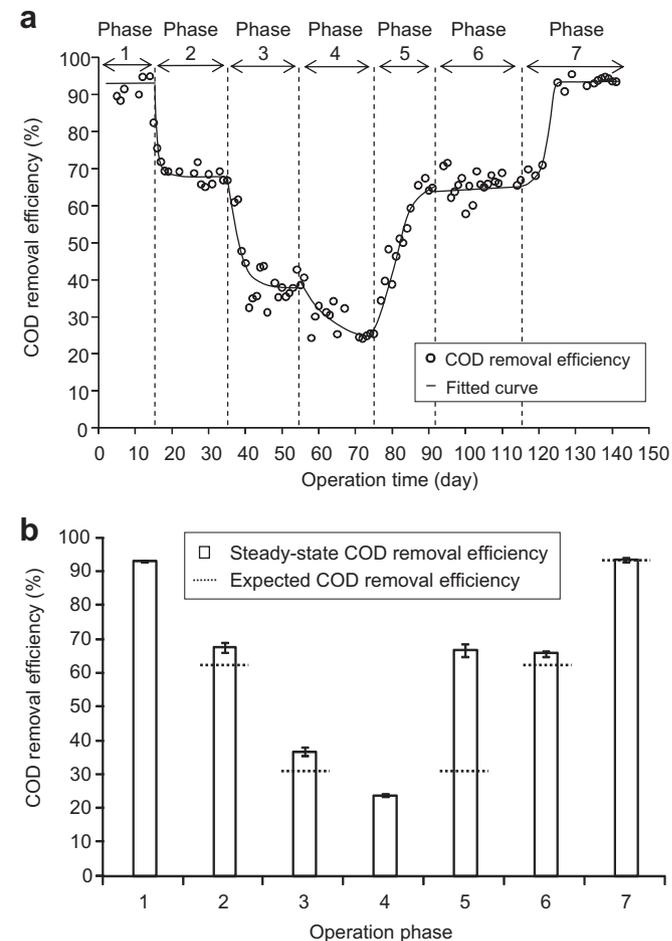
**Fig. 2.** (a) COD removal efficiency in the co-digestion experiment using the upflow anaerobic sludge bed reactor. (b) Steady-state COD removal efficiency (white bars) and the expected COD removal efficiency from synthetic wastewater based on the Phase 1 removal efficiency (dotted lines). Phases are described in Table 2. Errors are standard deviations.
