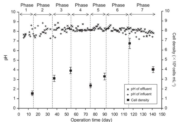
**Fig. 1.** pH and microbial cell density in the co-digestion experiment using the upflow anaerobic sludge bed reactor. Operational phases described in Table 2. Errors are standard deviations.
