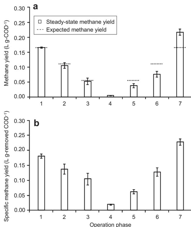
**Fig. 3.** (a) Steady-state methane yield (white bars) and expected methane yield from synthetic wastewater based on the Phase 1 yield (dotted lines). (b) Specific methane yield of each phase in the co-digestion experiment using the upflow anaerobic sludge bed reactor. Phases are described in Table 2. Errors are standard deviations.
