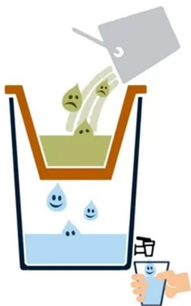
Figure 1. Conceptual representation of a ceramic water filter integrated into a safe storage container. Image courtesy of Potters for Peace ( pottersforpeace.org ).
